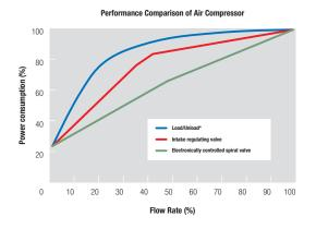
The main cost to operate an air compressor - is energy costs. The saving of the energy cost can recover from the initial air compressor investment. Effectively matching compressor production capacity with sprial valves to facilitate your needs and also the best way to save both energy and money.
